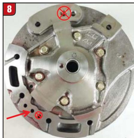
On a properly working torque converter you should not be able to turn the shaft while applying about 10-18 psi of regulated compressed air. If you want to see a video of this go to [Valvebodypros.com](http://Valvebodypros.com) and under the Support tab click on Pro Tech Tips, then click on Video.
