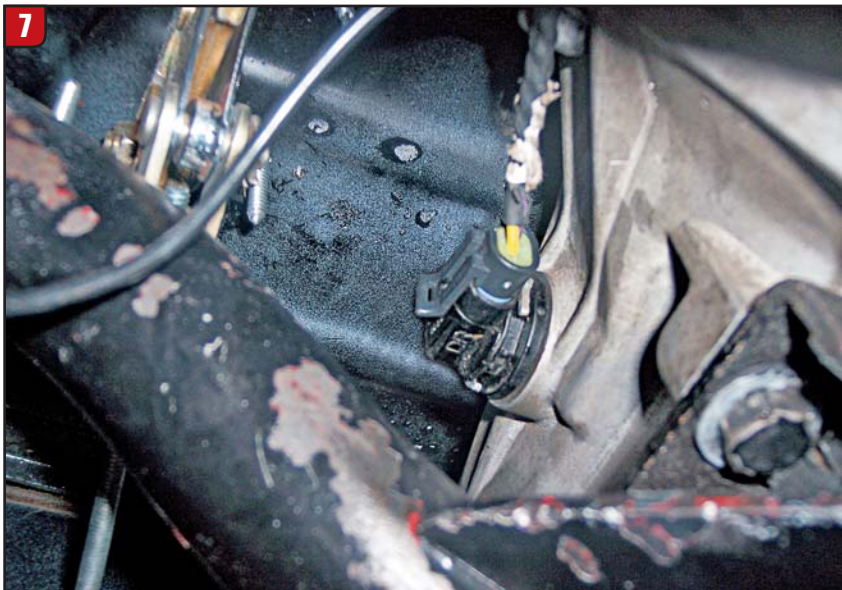
VSS pointing toward front of car
