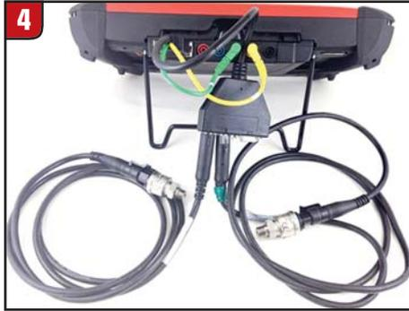
Two pressure transducers connected to a dual-channel graphing meter
