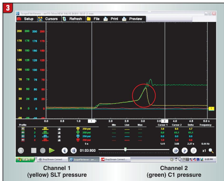
until the air pressure reached a certain point, and then the piston would apply immediately.
